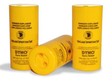
The TROJAN SPARTAN SR (Shock Resistant ) cast booster also incorporates the unique Caplock™ feature which holds the detonator in place more securely and makes it more difficult for the detonator to be pulled out of capwell position while it is being lowered into the borehole. Even with this new Caplock feature, the detonator can still be removed if necessary.
